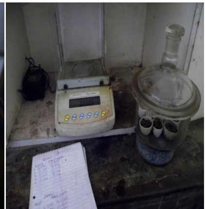
Samples in crucibles being weighed
