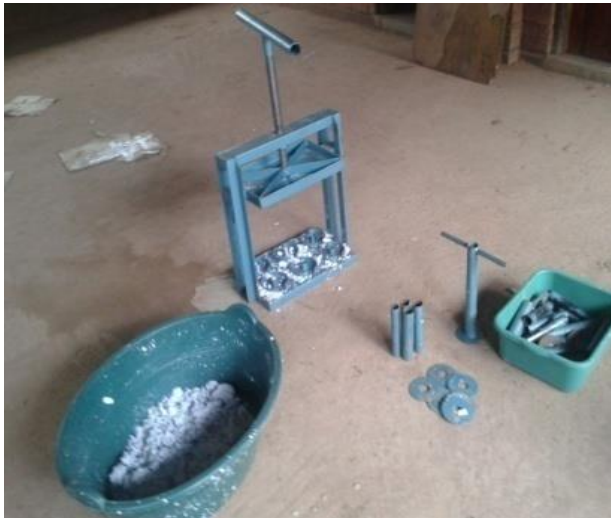
Figure 3: Screw Briquette making machine and its componets
