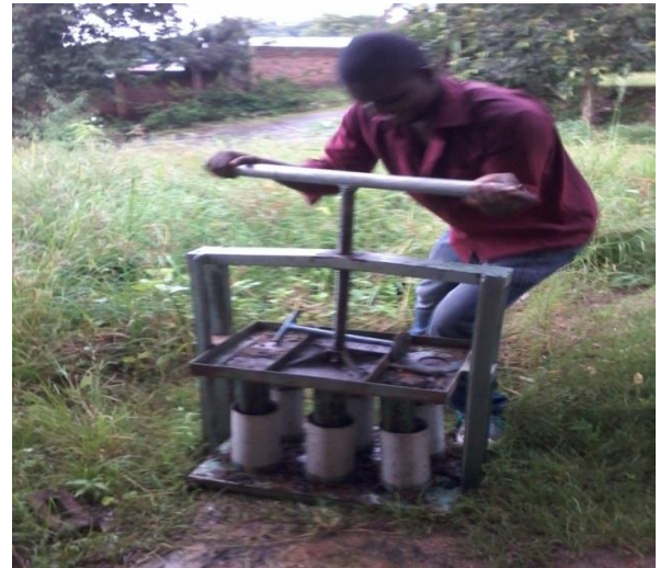
Figure 4: Compressing the mixed sawdust-banana peeling pulp
